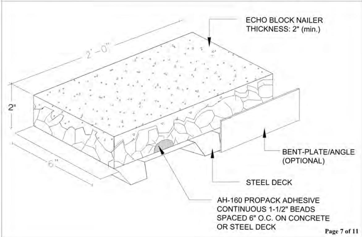
**ECHO BLOCK NAILER 6" WIDE x 24" (2" to 10" HIGH) OR ECHO BLOCK 24"x24" PER WATERPROOFING NOA**
